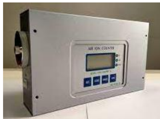
Figure 6: COM 3200 Pro II ion meter used for ion measurements of the PA663 ionizer.
