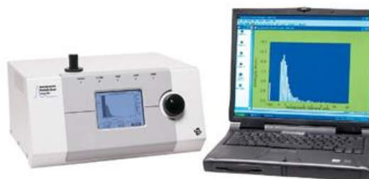
Figure 9. TSI Aerodynamic Particle Sizer (APS) model 3321 used to measure total particle concentration and particle size distribution of the challenge bioaerosol. It has a range of 0.54-20.0 μm aerodynamic diameter, with 1 particle/L detection limits.
